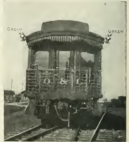
FIG. 2. MARKER LIGHTS, GREEN TO REAR WHEN ON SIDING TO BE PASSED BY TRAIN RUNNING IN SAME DIRECTION.
